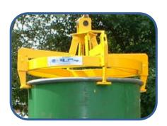
Our Drum Tongs are used for picking up 210 litre drums of the tight head or open topped steel varieties. The tongs can be fitted under a fork mounted hook, fork or carriage mounted jib, or under an overhead or lorry mounted crane. Semi-automatic in operation.
