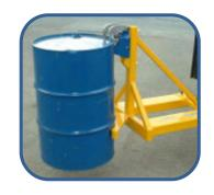
Our Rim Grip Drum Handlers offer fast and safe movement of drums via hardened steel jaws that grip the drum chimb (rim), allowing the drums to be picked up/set down with minimal gap between them. Ideal for stuffing/de-stuffing containers, suitable for use also on rough terrain. May be used for use with 120 or 210 litre Steel Drums and "L"/"XL" Plastic drums. A Spark Proof model is available for Zone 1 conditions. Not for use with empty drums
