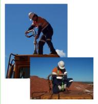
Access to maintenance areas on **Mobile Plant** provides specific access needs. Standard fall protection often wont work due to the low clearance allowances. The fact that this maintenance is required anywhere on site during a failure compounds the problem.
