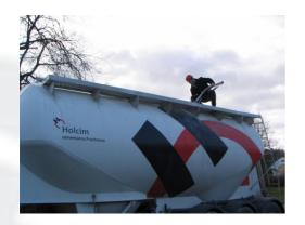
Access to maintenance areas provides specific access needs. Standard fall protection often wont work due to the low clearance allowances.
