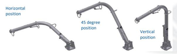
**The Fixed Base TRAM** consists of a pivoting TRAM Arm without a TRAM Rail. This gives the operator access and egress from a ladder to a platform where movement by the operator long a fixed rail is not required. A 270 degree rotating arm may be fitted to provide access to a greater work area.
