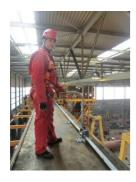
**Site Installed** cranes often have height restrictions for access areas on the top side of the boom, where motors and cable drums are housed. This removes the possibility of hand rails and other such passive safety systems.
