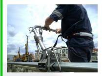
Access to maintenance areas on **Drill Rigs** provides specific access needs. Standard fall protection often wont work and the **TRAM** system is ideal for this situation, with stainless steel construction and robust manufacture.
