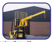
to be slung at greater centres than with conventional fixed jibs. The greater length available allows loads to be picked up from otherwise inaccessible areas. Supplied with two swivel hooks. This jib is *Manual Extension*.
