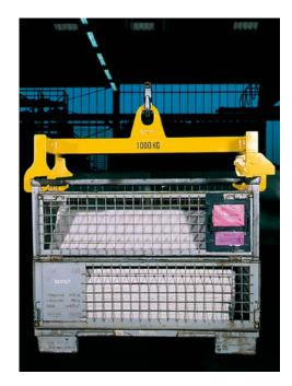
When using these spreader beams, it is important that the hooks be fastened only to the top frame of the box pallets.
