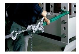
All ratchet lever hoists can be used for load attachment according to EN 12195.
