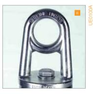
Unieye end anchorage connector – 316 stainless steel casting (electro-polished), 100% x-ray & die penetration inspection, 67kN (14,773lbs) breaking strength, Individual serial numbers for traceability, allows free movement of the system terminations thereby preventing dangerous leverage to the clevis
