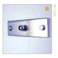
Wall Anchor Plate – 316 stainless steel, electro-polished. 50kN (11,205lbs) min breaking strength. 2 x M12 fixing holes
