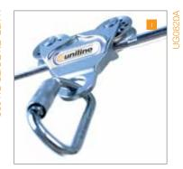
Attachment Carriage – Single user attachment, 17/4PH stainless steel casting – very strong, 100% x-ray and die penetration inspection, electro-polished for long term corrosion resistance, individually serial numbered for traceability, sealed bearings for smooth running and functionality, passes freely over intermediate brackets
